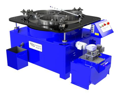
The Lapmaster Model 48 is equipped with a 48 inch (1219mm) diameter lap plate. This is manufactured from Grade 300 grey cast iron to ISO 185(2005). It consists of individual segments bolted to a support plate.
